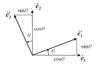
Figure 3. A rotation in the plane. The physical vectors  $\hat{e}_1$  and  $\hat{e}_2$  are the prior basis, and the physical vectors  $\hat{e}'_1$  and  $\hat{e}'_2$  are the posterior basis.  $\theta$  is the angle of rotation, and the physical axis of rotation is  $\hat{e}_3$ , which is the same as  $\hat{e}'_3$  (neither shown).
