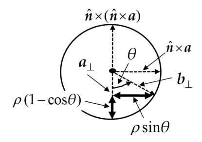
Figure 2. A physical rotation as seen in the tangent plane.  $\theta$  is the angle of rotation, and  $\hat{n}$  the physical axis of rotation. The prior physical vector is a, and the posterior physical vector is b. The subscripts  $\parallel$  and  $\perp$  denote components parallel and perpendicular to  $\hat{n}$ , respectively. The quantity  $\rho$  is equal to  $|\hat{n} \times a|$ .
