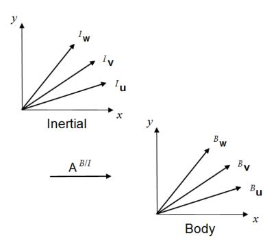
Figure 5. Transformation of inertial representations to body representations. The upper diagram shows the inertial representations of the physical vectors u, v, and w, while the lower diagram shows the body representations of the same physical vectors. A <sup>*B*/*I*</sup> is the attitude matrix that transforms column-vector representations from the inertial frame to the body frame.
