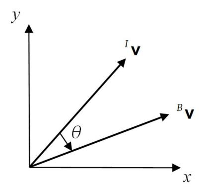
Figure 4. Two column-vector representations.  ${}^{I}\mathbf{v}$  and  ${}^{B}\mathbf{v}$  are the representations of the physical vector  $\mathbf{v}$  with respect to the inertial and body frames, respectively. The basis of the inertial frame is the same as  $\mathcal{E}$  in Figure 3, while the basis of the body frame is the same as  $\mathcal{E}$ ' in Figure 3.
