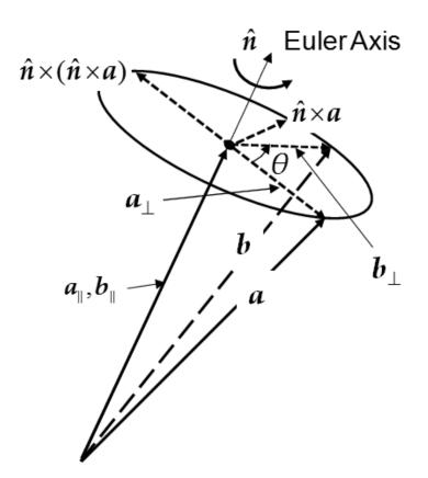
Figure 1. A physical rotation in three dimensions.  $\theta$  is the angle of rotation, and  $\hat{n}$  the physical axis of rotation. The prior physical vector is a, and the posterior physical vector is b. The subscripts  $\parallel$  and  $\perp$  denote components parallel and perpendicular to  $\hat{n}$ , respectively.
